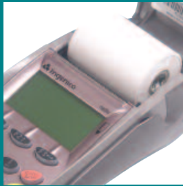
Easy load 15 lines per second thermal printer
